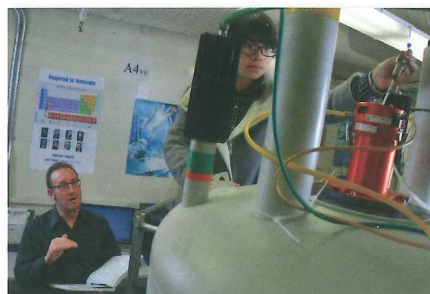
Ying inserting an ion gel sample into the NMR spectrometer for analysis
